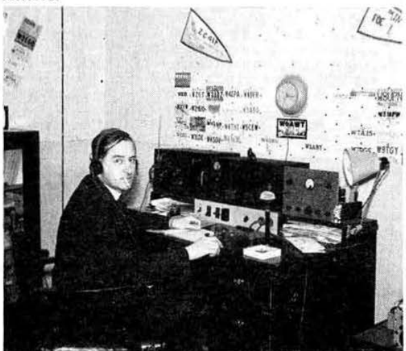
Third in the 1957 B.E.R.U. Contest was ZC4IP of Limassol, Cyprus. In this picture, the BC221 frequency meter is to the left of the 1936 vintage HRO receiver and a home-built 85 kc/s i.f. unit to the right.
