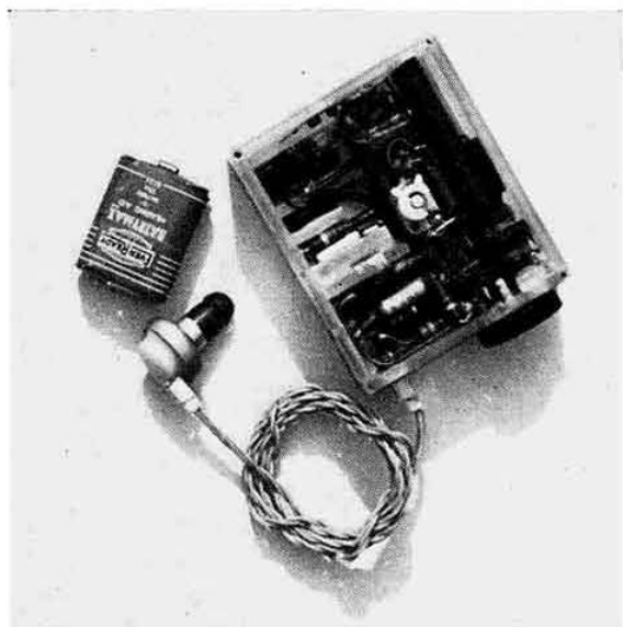
The miniature receiver with the battery removed. Its size can be judged from the earpiece.
